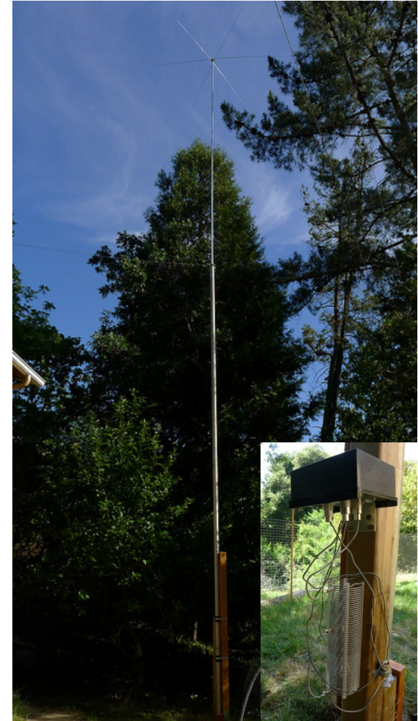
Increased 33' vertical to 45' w/six 5' top hats, added Switchable Base LC's
